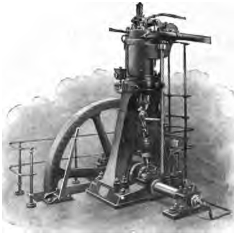
SINGLE CYLINDER DIESEL MOTOR, 20 H. P.
